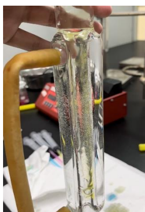
Fig. 5. The flowing distance and gelling time test of MC/HA-Me hydrogels by a condenser tube simulated.
