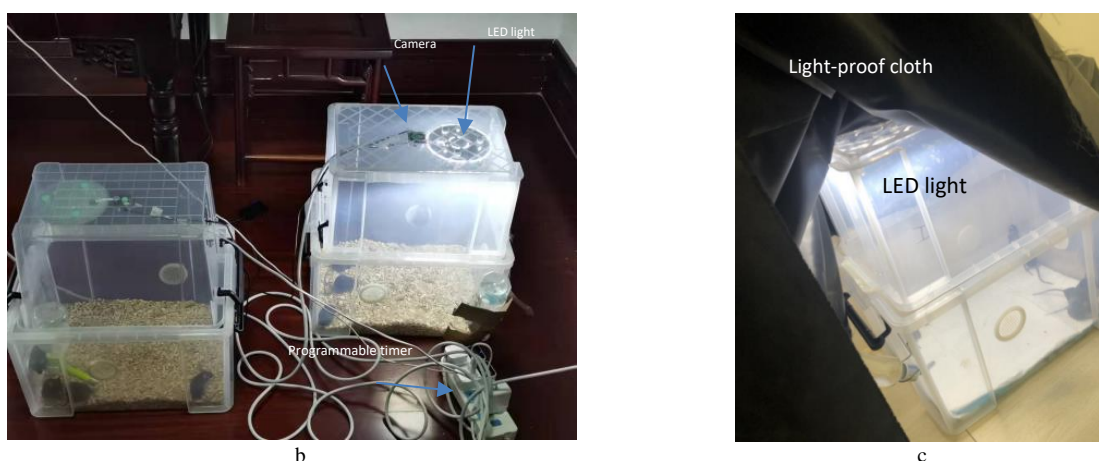
Fig. 3. Circadian rhythm induction chamber. a: Schematic diagram of the mouse colony and circadian rhythm induction chamber setup. b: Photo of the custom-built circadian rhythm induction chamber housing 4–5 mice in a light-proof cage at room temperature. c: Light-proof cloth completely covering the cage.
