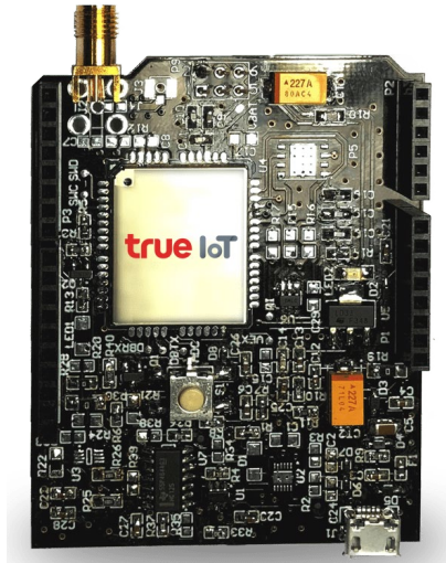
Figure 4. NB-IoT shield board.
