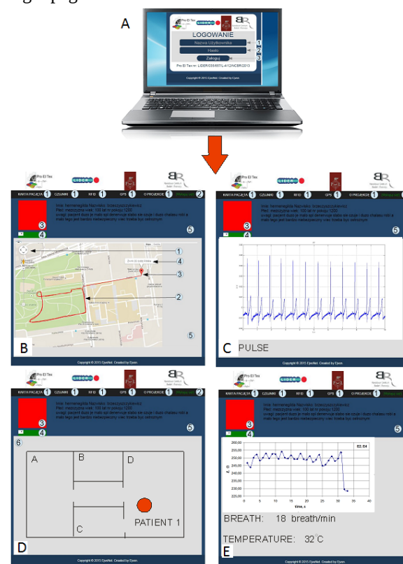
Figure 21. The structure of a software for monitoring patients
