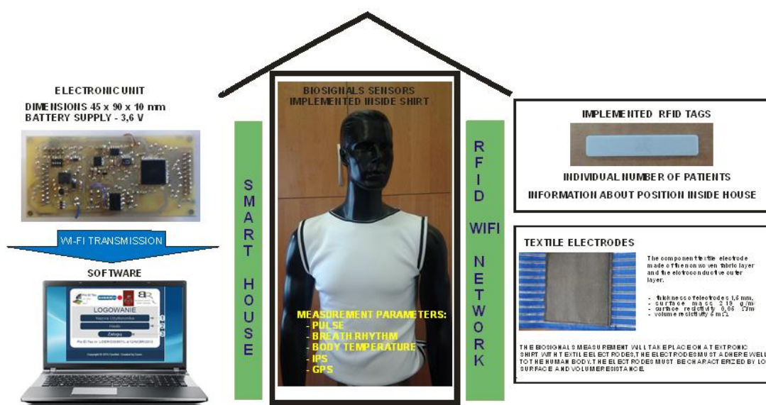
Figure 3. The scheme of the textronics system for protecting of elders
