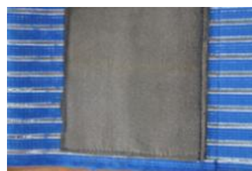
Figure 5. The component textile electrode made of the nonwoven fabric layer and the electrically conductive outer layer
