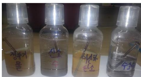
Figure 12. An experiment comparing corrosiveness of iron nails in solutions mixed with various gases
