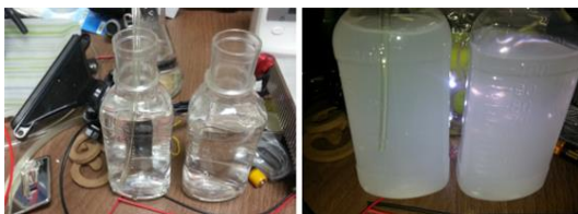
Figure 17. Solubility observation experiment after producing hydrogen for 10 minutes (left) and applying pain painkiller pill (right)
