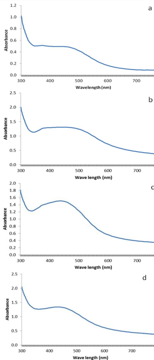
Figure 1. AgNps synthesis by *B. licheniformis* a)1mM b) 3mM silver nitrate solution with supernatant, c)1mM b) 3mM silver nitrate solution with biomass.
