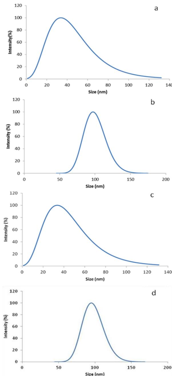
Figure 3. Size of AgNPs synthesized by *B. licheniformis* a)1mM b) 3mM silver nitrate solution with supernatant, c)1mM b) 3mM silver nitrate solution with biomass
